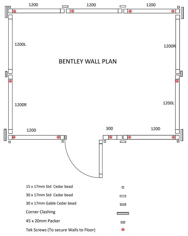
Please note: The walls are not screwed down to the floor until all the walls are erected, the roof is in place and the doors are about to be installed.
