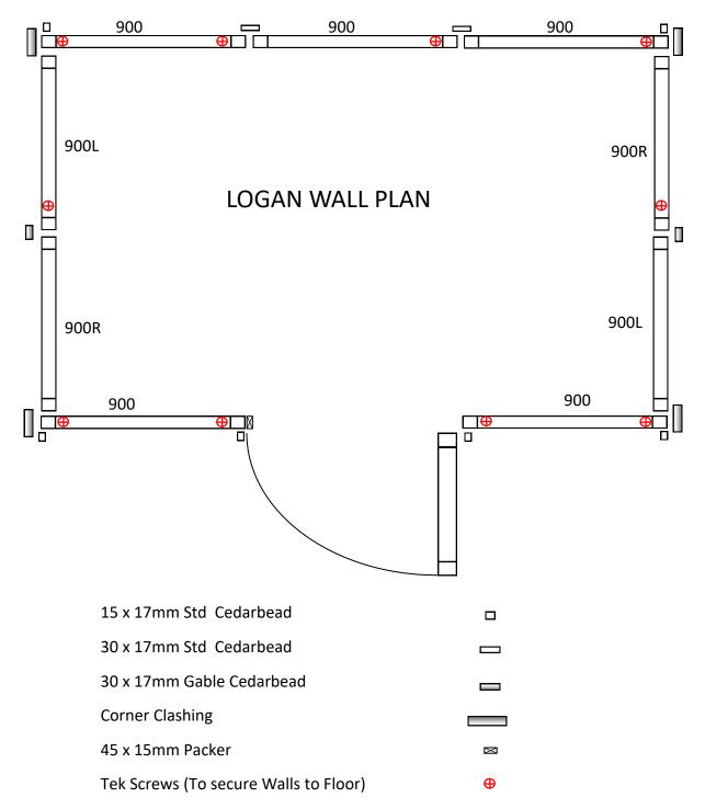
Please note: The walls are not screwed down to the floor until all the walls are erected, the roof is in place and the doors are about to be installed.
