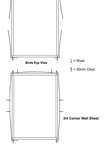
**Step 4:** Nail Wall Sheets to Plates, two 30mm Clouts per pan top and bottom. Nail Wall Sheets to Wall Nogs, one clout per pan.
