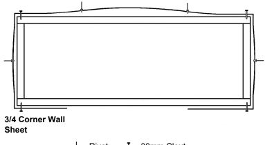
**Step 4:** Nail Wall Sheets to Plates, two 30mm Clouts per pan top and bottom. Nail Wall Sheets to Wall Nogs, one clout per pan.
