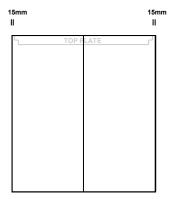
Standard Shed — Bottom Plate will protrude below wall sheet by approximately 10mm.
